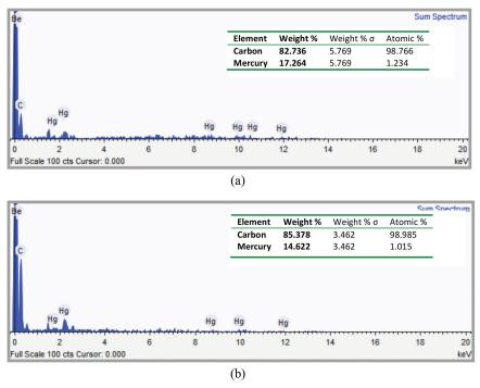
FIGURE 4. Energy-dispersive X-ray spectroscopy analysis of activated carbon after adsorption: (a) 50 mg/L of Hg(II) initial concentration and 20 mL/min of flow rate; and (b) 100 mg/L of Hg(II) initial concentration and 20 mL/min of flow rate.
