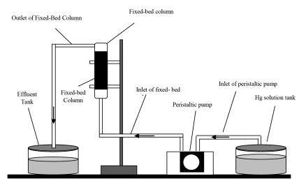
FIGURE 1. Schematic experimental set up of the adsorption process
